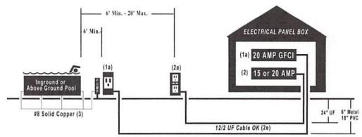
MUST BE THWN, etc #12 WIRE IN CONDUIT (no UF cable) (1d)
